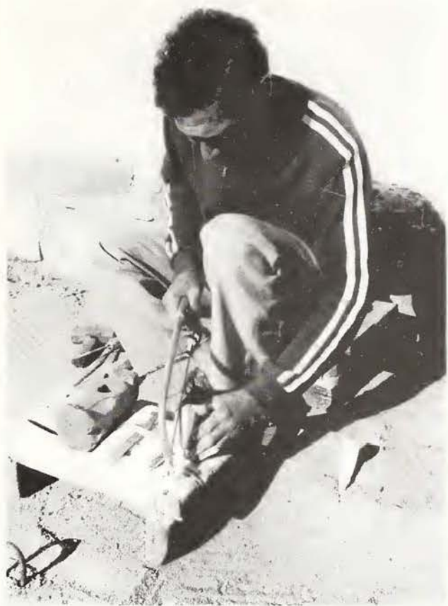
Fig. 1. E uses a saw to produce the rough shape of the pipe.
